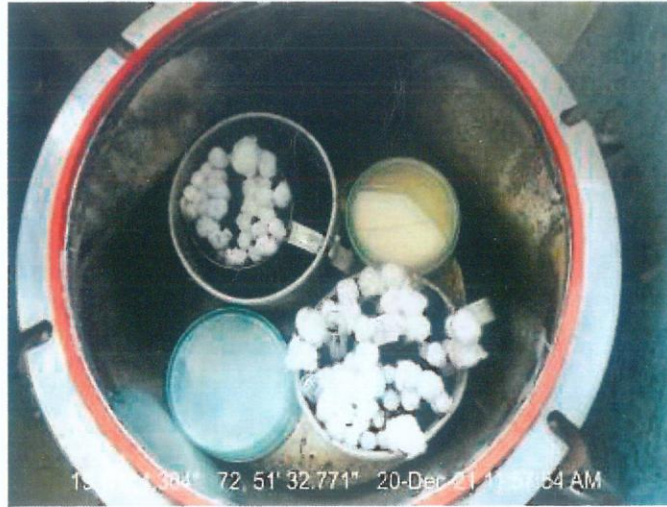
Discarded media and microbial cultures from experiments in the Microbiology laboratory in a small autoclave before sterilization
